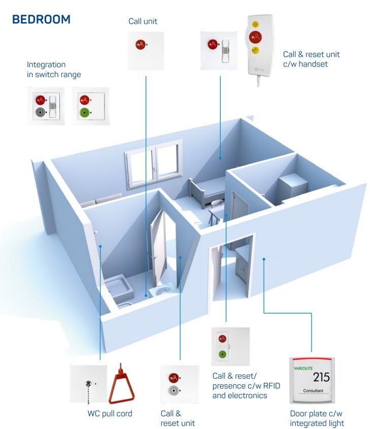
The visually appealing display elements in the corridor and the possibility of integrating the call units into switch ranges increase living comfort. At the same time, the high security standard of the call system is maintained at all times.
