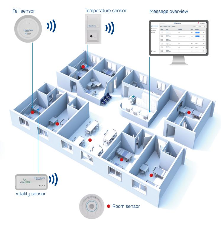
A variety of different sensors automatically collect care data and transfer it directly to the existing care software. In addition, automatically generated alarms are transmitted directly to the call system. This ensures that nursing staff are kept informed at all times. Work routines can be made more efficient and the quality of care is improved thanks to shorter response times.
