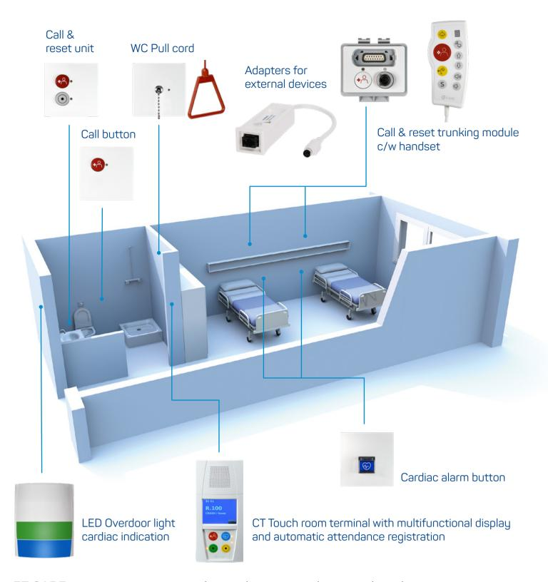
**EZ CARE** room components can be easily integrated into modern day care environments. The modular system offers the right solution for every requirement – for example, seamless integration into a bedhead trunking.
