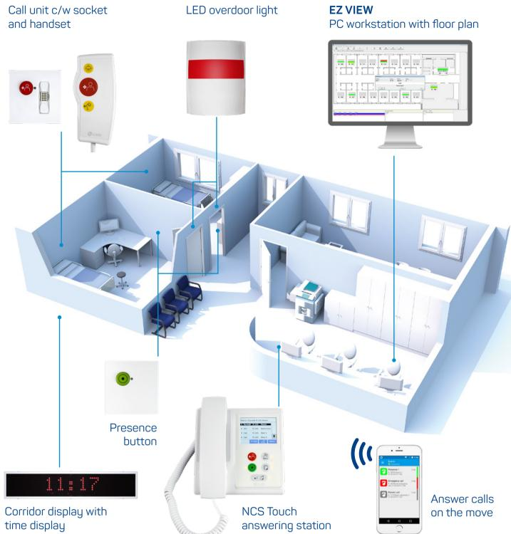
A variety of different displays are available for the nurse base. Receiving and managing calls is facilitated by EZ CARE displays. There are many ways to do so in easy, intuitive and time saving ways. The integrated speech supports the
