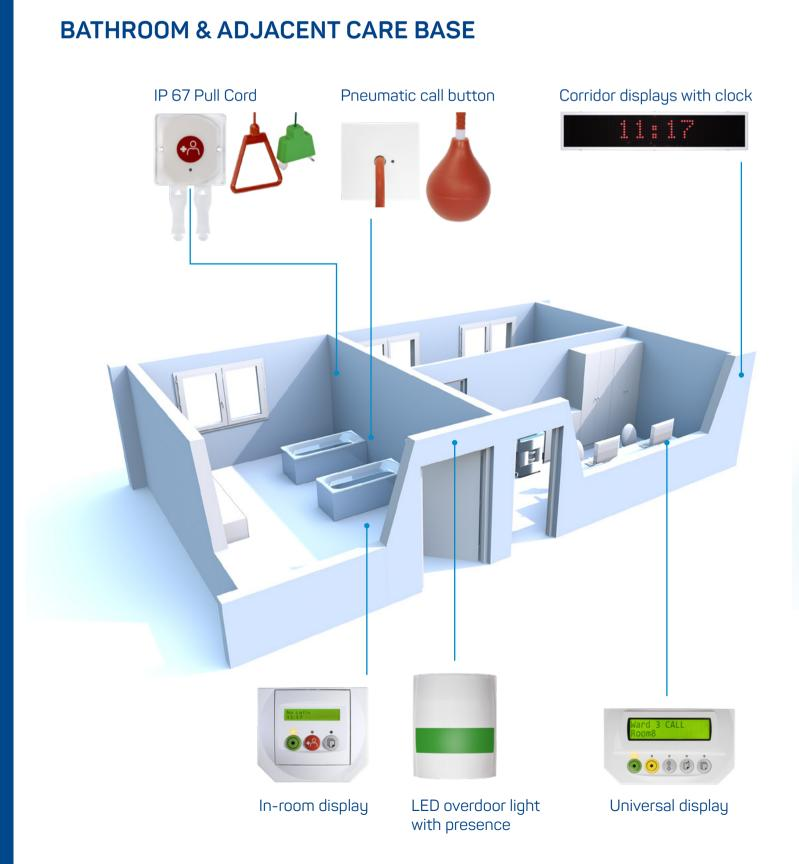
EZ CARE universal displays are used to display and manage calls where no speech is needed. In particularly demanding environments – for example the bathroom – special units such as pneumatic call button or waterproof pull cord are used.
